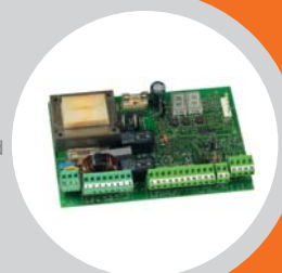
455D control board
